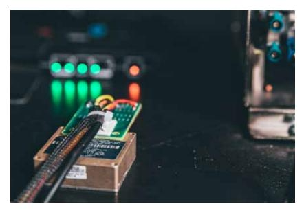
needs to have as much intelligence as possible to understand where it is....The IMU helps reduce the error rate and maintain a trajectory that's closer to ground truth."
